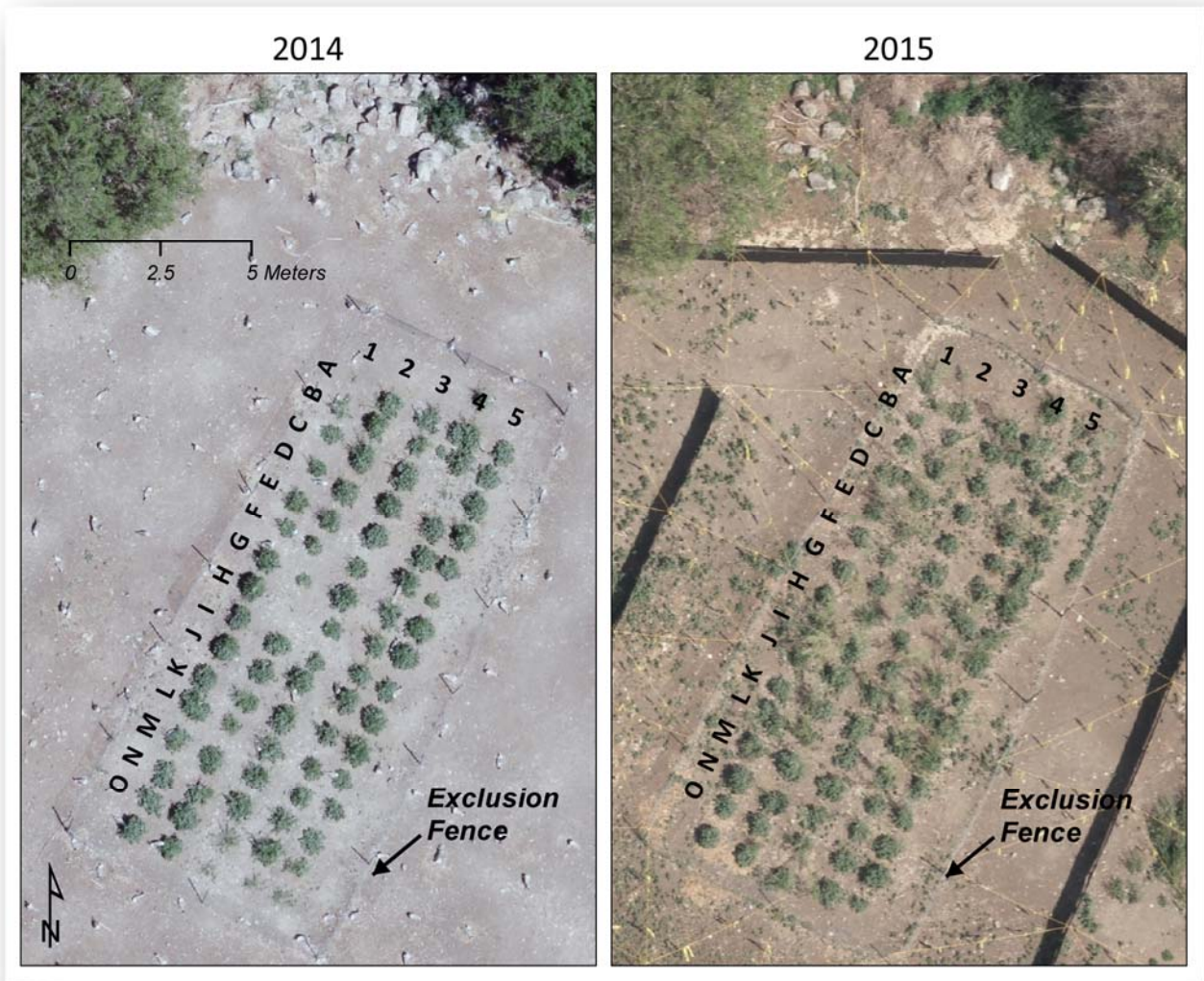
Map 9. Aerial image of the willow test plot on Crescent Island, mid-Columbia River in May 2014 and May 2015. Vegetation growth inside the plot includes planted native willows as well as non-native annuals. Holes for 75 individual plantings were drilled 3-4 feet apart in five columns (numbered 1-5 from east to west) and 15 rows (lettered A-O, running downslope from the island's edge). An exclusion fence was installed around the plot to protect the willows from browsing mammals.
